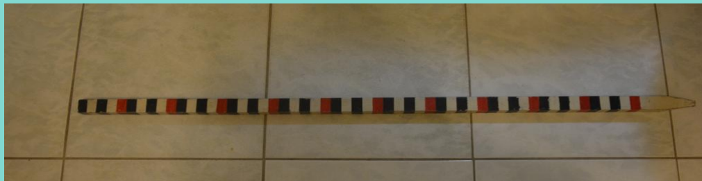
Figure 7-1 The "Emery board" apparatus for measuring beach profiles, consisting of two wooden boards marked from the top with rulers to measure the distance a , which is equal to the beach elevation change b . The length of the rope controls the measurement interval.
